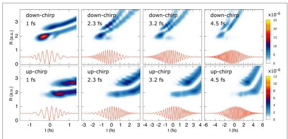
**Figure A2.** Nuclear wave packets pumped into the  $3p\sigma_u$  state for different chirped pulses (plotted in red lines). Upper panels: negatively chirped pulses. Bottom panels: positively chirped pulses.
