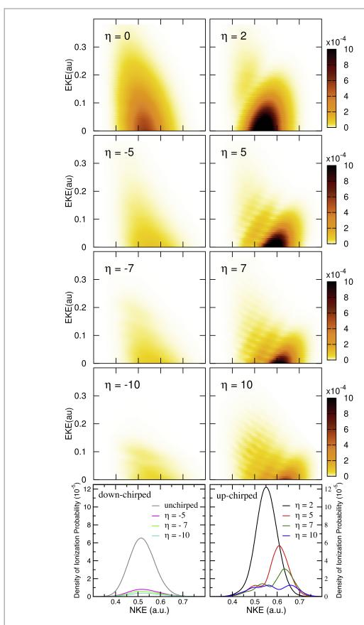
**Figure 4.** Panels in the four upper rows: electron (*y*-axis) and nuclear (*x*-axis) energy differential two-photon density of ionization probability, i.e. fully differential energy distribution for the ionized fragments after Coulomb explosion for different values of the chirp parameter as indicated in each subplot. Bottom row: corresponding nuclear energy distributions resulting after integration over electron energy (the value of the chirp parameter is indicated in the legend).
